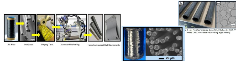
Figure 1. Spool and electron microscope image of GA-EMS produced 2.9 GPa SiC fiber
