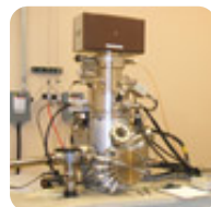
Scanning Auger Nanoprobe
